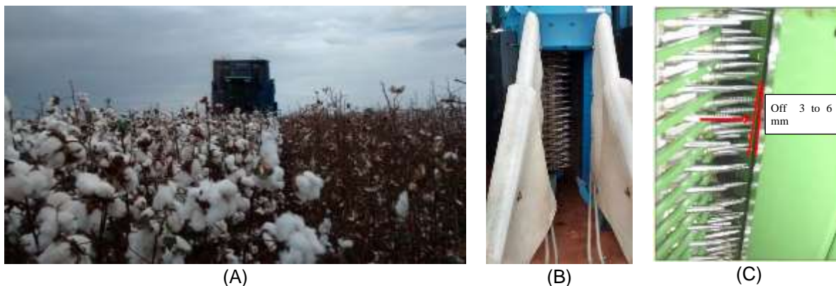
Figure 1. Harvester (A) harvesting unit (B) and adjustment of the nip pressure plate (C).
