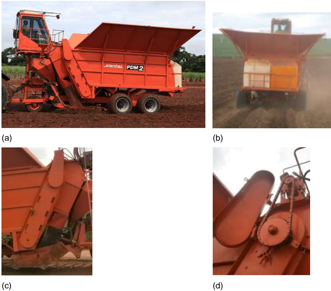
Figure 1. Sugarcane billet planter (a and b); billet metering system (c and d).
